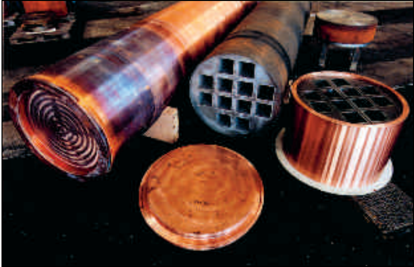
Figure 4.2 Example of manufactured canister components: copper tube, cast iron insert and copper lid.
